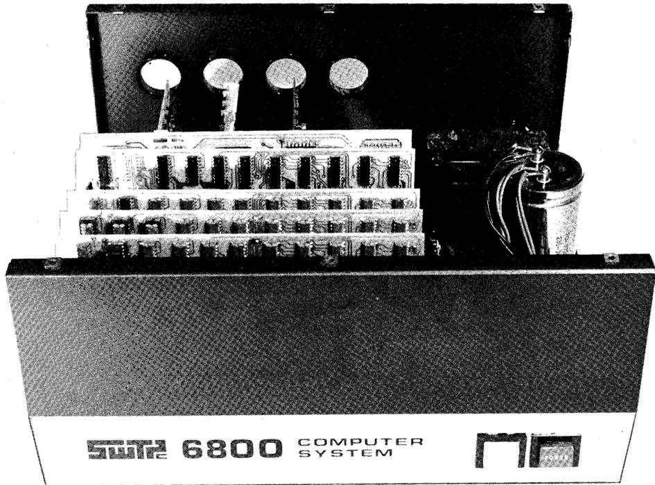
Figure 1-7 Southwest Technical Products' 6800-based personal computer system.
