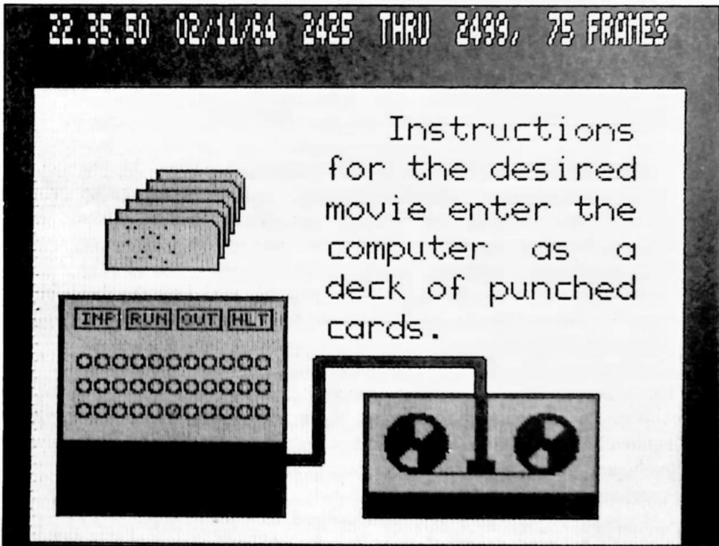
Fig. 8-3. Animated movies by computer have been developed by Bell Telephone Laboratories. The computer, programmed in BEFLIX language, generates a tape; the tape is fed to a General Dynamics Microfilm Recorder that produces a picture on the face of a cathode ray tube. These images are photographed, and make up the frames of the film.
